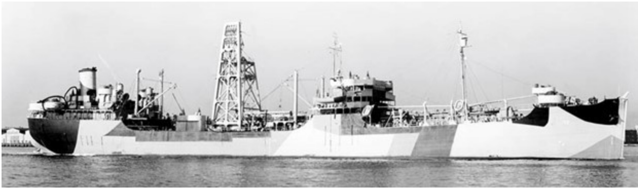
Caption: Niobrara in wartime camouflage at Norfolk, 18 April 1944, before departing for the Pacific, showing the 160-ton capacity derrick installed to facilitate the handling of tank landing craft (LCT) to tank landing ships. (U.S. Navy Photograph 19-N-64643, National Archives and Records Administration, Still Pictures Branch, College Park, Md.)
